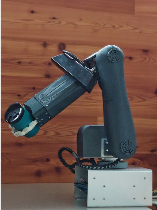
Figure 2: The finished robotic arm holding a cup.
